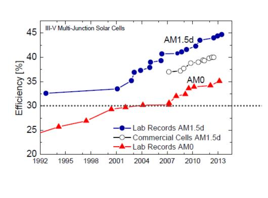
Efficiency of 3-junction solar cell under AMO (Space solar cell)
